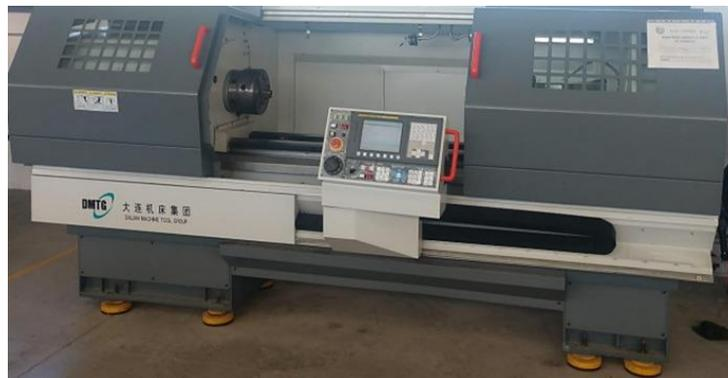
**Figura 15.** Torno CNC DMTG CKE 6150Z.
